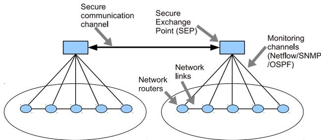
Fig. 1: P3CA system architecture.
